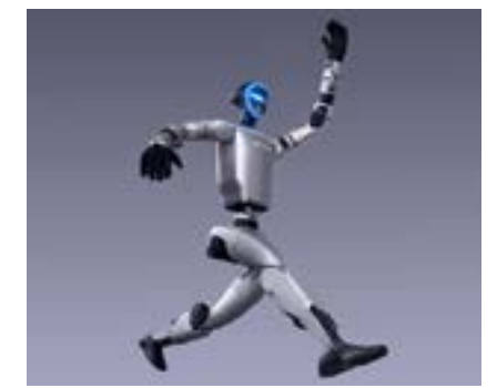
28 Unitree G1 Humanoid Robot, 2024, Unitree Robotics, Aluminum alloy + plastic + electronic components, 51" x 18" x 8"
