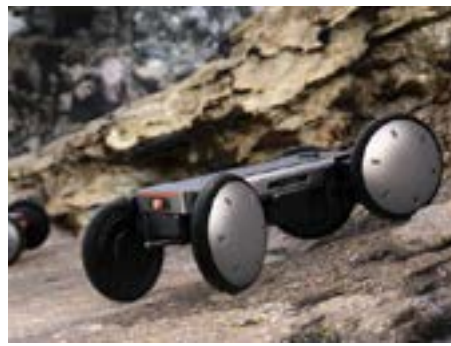
31 Hyundai MobeD Autonomous Robot Platform, 2026, Hyundai Motor Group, Aluminum + electronic components + sensors, 25" x 24" x 18"
