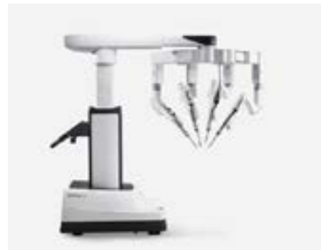
60 Da Vinci Xi Surgical System, 2014, Intuitive Surgical, Stainless steel + aluminum + plastic + precision actuators + electronic imaging systems, 69" x 49" x 87"
