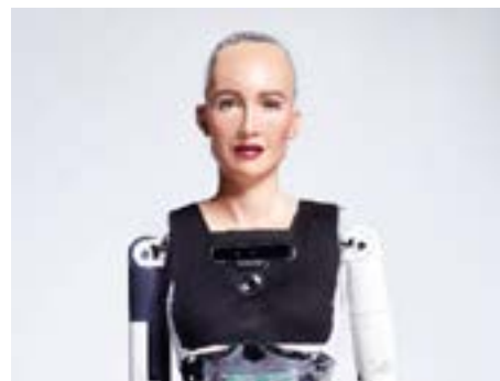
12 Sophia Humanoid Robot, 2016, Hanson Robotics, Silicone + plastic + aluminum + electronic components, 67" x 24" x 20"
