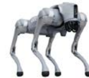
03 Unitree Go2 Robodog, 2023, Unitree Robotics, Aluminum alloy + plastic + rubber + sensors, 16" x 11" x 20"
