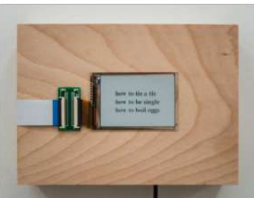
085 how to..., 2015/2016 Zach Gage, Custom wood enclosure, raspberry pi, adafruit pervasive visions 2.7" display kit, ribbon cable extender, 5 x 7 x 2 in
