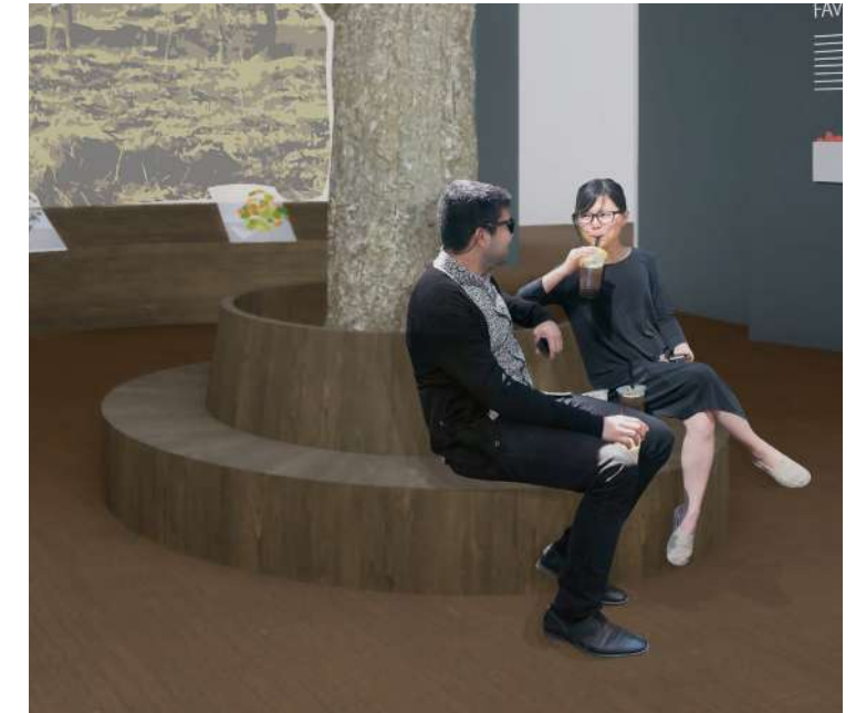
CIRCULAR BENCH Dimensions: 10'8" x 10'8" x 1'6"-3'3" Material: M-1 Oak Features: Curved 360 design allows visitors to view any angle of the exhibition Quantity: 1 Location: Main exhibition space around tree sculpture
