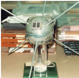
CL001 Satellite Vanguard 1 Replica Materials: Aluminum Dimensions: 6 in. diameter (15.2cm); the antennae fit within a 2 foot spherical volume
