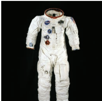
GL001 Pressure Suit, A7-L, Collins, Apollo 11, Flown Dimensions: 5ft 6in. x 2ft 8in. x 11in. (167.64 x 81.3 x 27.9cm) Materials: Exterior: Beta cloth, nylon, polyester, velcro Interior: Neoprene/Rubber, nylon
