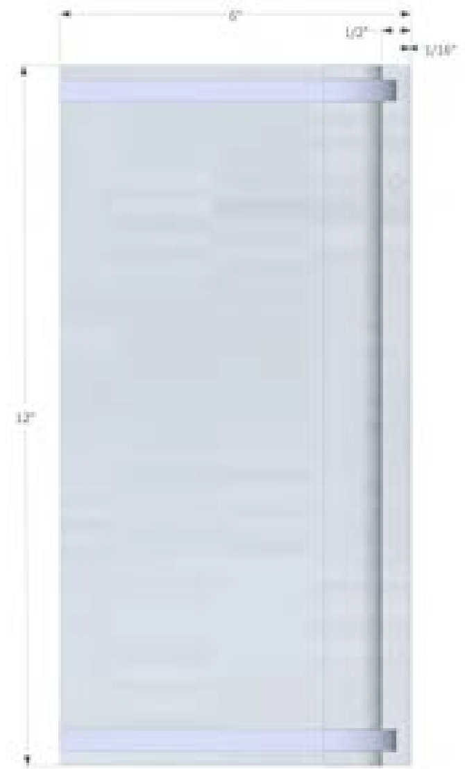
FRONT ELEVATION Note 3/8" groove machined on top and bottom to allow for insertion of case panels, holes for pins to join panels together.
